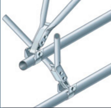
With the TwinCabrio rail mechanism, the two window push rods run through each other (on the lower and upper push-pull tube, respectively). A unique calculation programme (commissioned by Van der Valk Systemen and developed by TNO Bouw) precisely calculates the space they require for each situation. Friction is eliminated and operational safety guaranteed.
